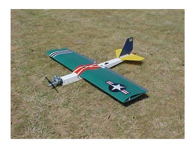
This little gem is named the Debut - and like its name implies - it is designed as an introductory, beginners RCCA open "B" class plane. With a whopping 48" streamer grabbing wingspan, and an all up flying weight of just slightly over 3 lbs (with full size radio gear and a Thunder Tiger Pro .25) this plane is a terrific entry level combat plane that can help you "learn the ropes" of combat!
