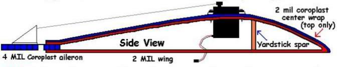
Note: Aileron hinge created by cutting away one side of a Coroplast corrugation
