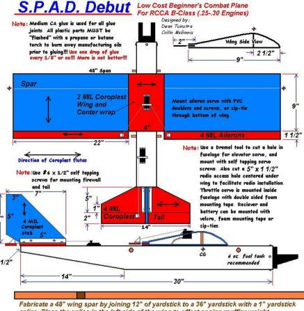
splice. Place the splice in the left side of the wing to offset engine muffler weight.
